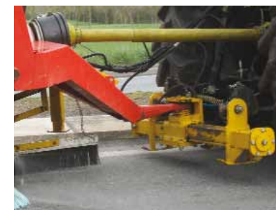
Special hook for side-shifting
